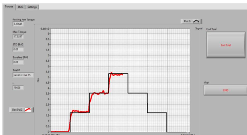
**FIGURE 2** Real-time on-screen biofeedback shown to the subjects during a representative trial. Black solid trace is the target torque, red solid trace is the subject's torque output.
